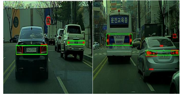
Figure 5. Final detected vehicle rear-lamp
