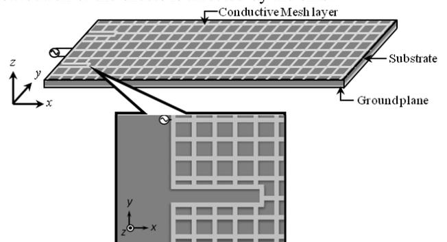
Figure 1. Geometry of proposed two-dimensional communication sheet
