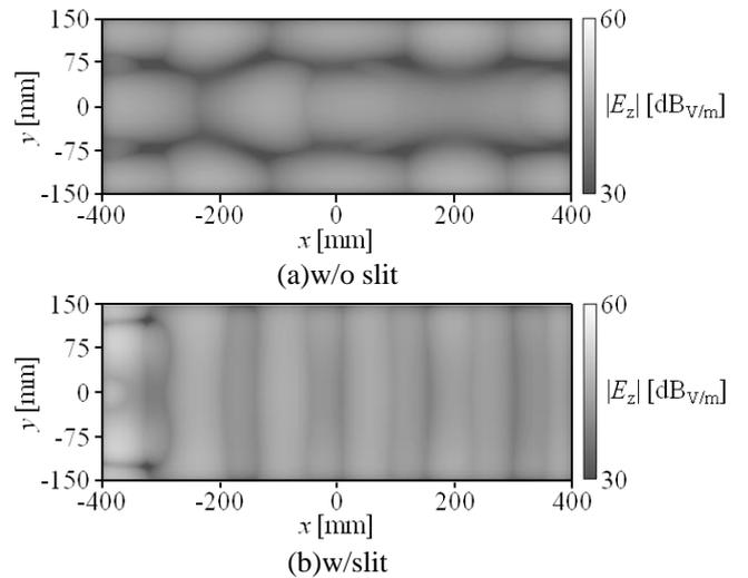
Figure 4. received  $|E_z|$  distribution of the sheet using diversity reception
