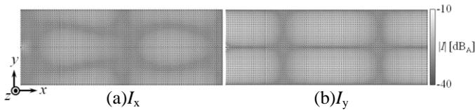
Figure 6. current distribution of the sheet without slits
