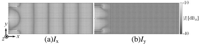
Figure 7. current distribution of the sheet with slits
