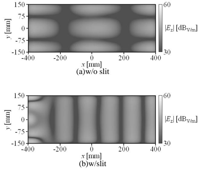
Figure 2.  $|E_z|$  distribution on the sheet with open termination
