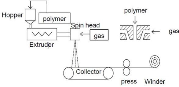
Figure 1. Meltblow technology to produce non-woven fabric.
