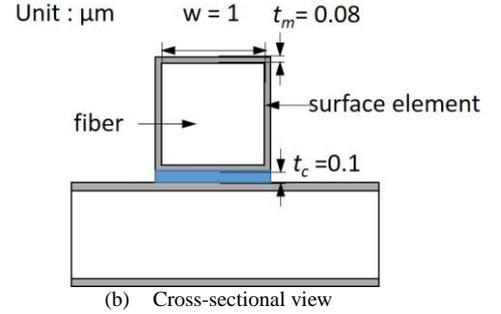
Figure 3. Thin fiber model with contact element
