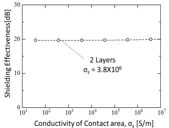
Figure 7. The contact area conductivity dependence of the SE with constant metal conductivity ( $\sigma_s=38 \text{ [S/m]}$ ).
