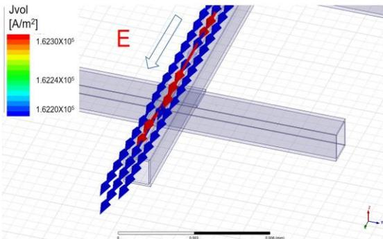
Figure 4. The volume current distribution of surface element around fibers with 90 degree electric field input.
