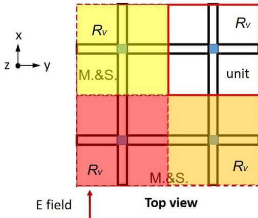
Figure 9. The definition of resistance in unit of 90 degree electric field input.
