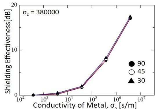
Figure 8. The conductivity of metal dependence of the SE with constant contact element conductivity in two layers model.
