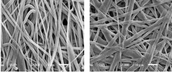
(a) Sample 1 (no heat treatment)      (b) Sample 2 (with heat treatment)
