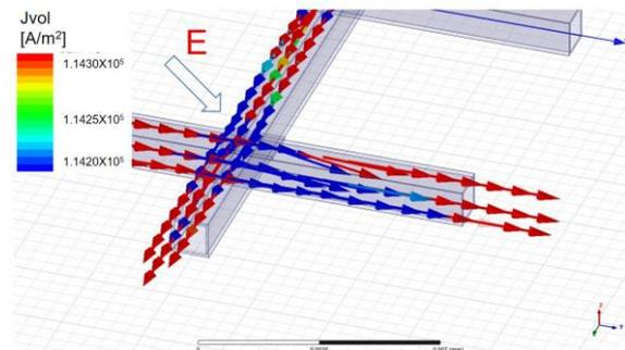
Figure 5. The volume current distribution of surface element around fibers with 45 degree electric field input.
