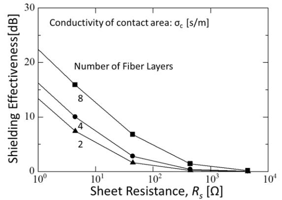
Figure 6. The sheet resistance of the SE with constant contact element conductivity ( $\sigma_c=38 \text{ [S/m]}$ ).
